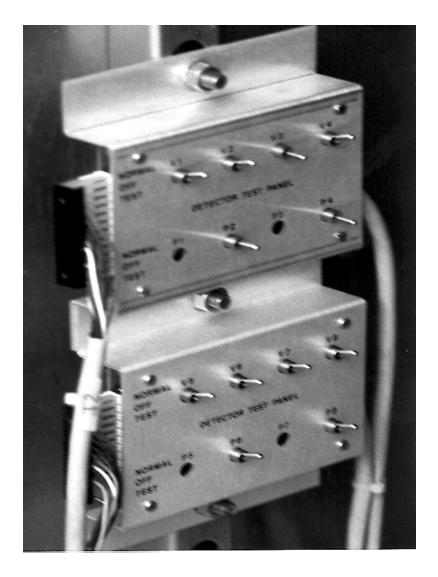
Each switch on the detector panel controls one phase. The switches can be turned off (so the phase never receives a call), can be left in normal operation, or can be used to place a test call on the phase. Activating the switch (or push-button) for a certain phase will place a test call on that phase for as long as the switch (or button) is held in the on position.
